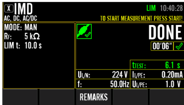
Figure 58: IMD (MAN mode) measurement result, example
