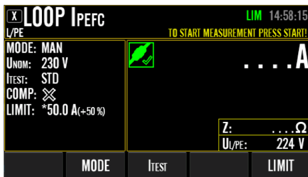
Figure 19: LOOP IPEFC (L/PE) idle screen with extended range of menu keys (after pressing "EDIT" menu key), example
