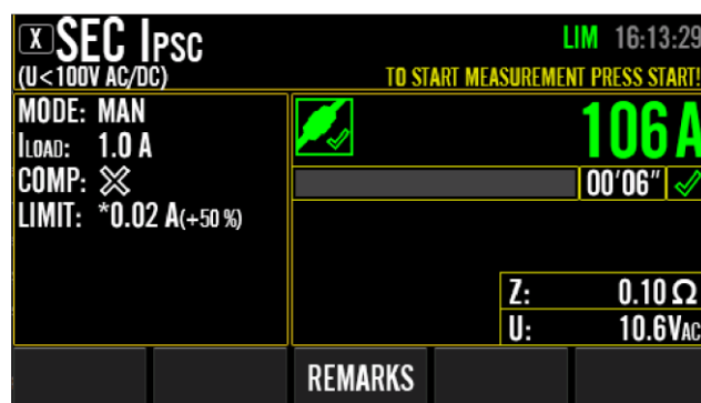
Figure 30: Final result in SEC IPSC ( U < 100V AC/DC) measurement, example
