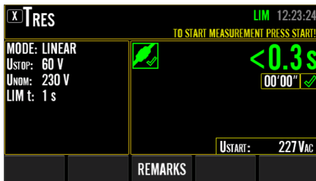
Figure 96: tRES measurement result in LINEAR mode, example
