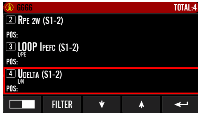
Figure 156. New created “MEMORY” with test steps copied from selected “TEST PLAN” Note!
