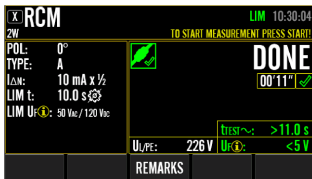
Figure 53: RCM (A type) measurement result, example
