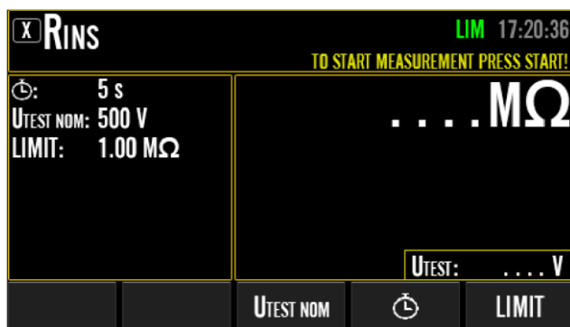
Figure 61: RINS idle screen with extended range of menu keys (after pressing “EDIT” menu key), example
