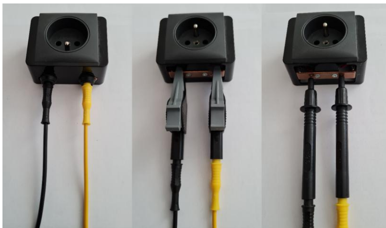
Figure 7: Connection of two test leads with banana (left figure), with test crocodile clip (middle figure) or with test tip (right figure) to Zero Adapter ZA-204-SC.
