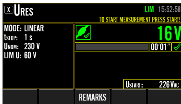
Figure 89: URES measurement result in LINEAR mode, example
