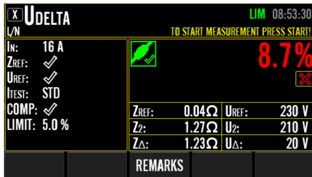
Figure 37: Final result in UDELTA measurement, example
