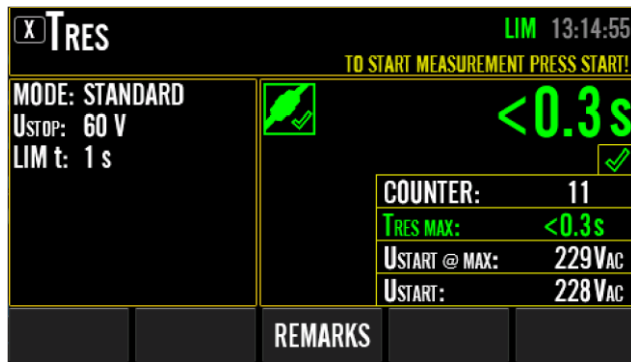
Figure 99: tRES measurement result in STANDARD mode, example
