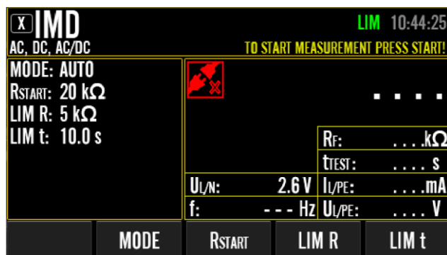
Figure 59: Idle screen in IMD measurement (AUTO mode) with extended range of menu keys (after pressing “EDIT” menu key), example
