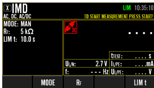
Figure 56: Idle screen in IMD measurement (MAN mode) with extended range of menu keys (after pressing “EDIT” menu key), example
