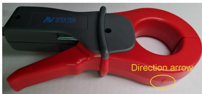
Figure 115: Direction marked on current clamp type CC-204-1000A
