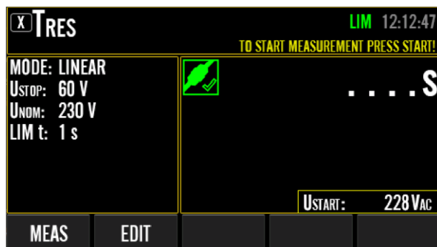
Figure 95: Idle screen in TRES measurement, example
