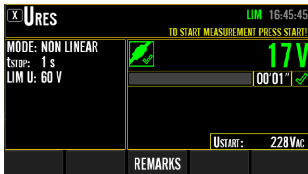
Figure 92: URES measurement result in NON LINEAR mode, example
